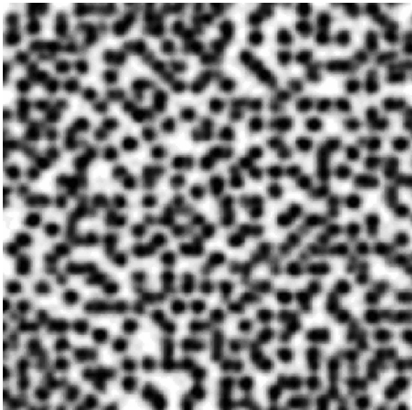
Figure 12. The enlarged central portion of a simulated microdischarge pattern in DBD. Simulation conditions are the same as for the experimental image in figure 10. The size of the microdischarge footprint is the same as in figure 10.
