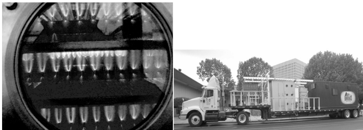
Figure 6. Large-volume, atmospheric pressure pulsed discharge plasma for treating VOC emissions. Left picture: discharge operation at 4 kW. Right picture: overview of the discharge system—pilot plant.
